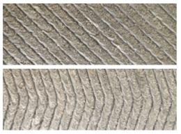
The 45 degree orientation of the welding bead to the conveying direction induces only small wear. Welding toes as well as hardening cracks are directed at a 45 degree angle to the conveyor stream, protecting the component against wear.
