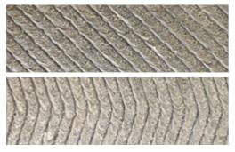
The 45 degree orientation of the welding bead to the conveying direction induces only small wear. Welding toes as well as hardening cracks are directed at a 45 degree angle to the conveyor stream, protecting the component against wear.
